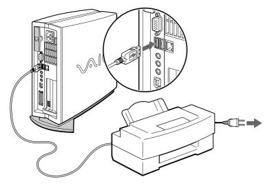
Do not turn on the computer or the printer until all the connections are made.
